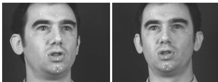
Fig. 1. Stereo images of one speaker, EK, with 15 markers on the face.
